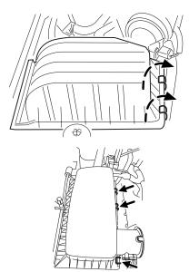
1. Release the clamps that secure the air filter housing cover. 324
